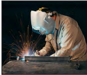
Conventional CV short circuit transfer using carbon dioxide (CO 2 ) and 0.045 in. solid wire.
