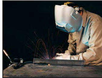
STT using CO 2 and 0.045 in. solid wire (Note reduced spatter and fume).
