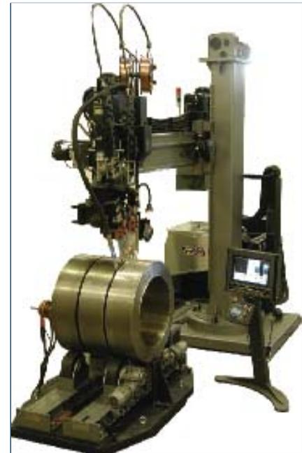
Fig. 8 — Integrated narrow groove welding system.
