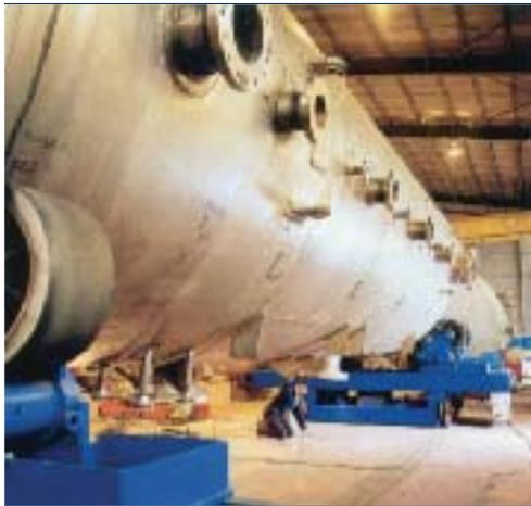
*The use of narrow, deep joints reduces the number of passes as well as the time and materials it takes to build pressure vessels such as the one shown above.*
