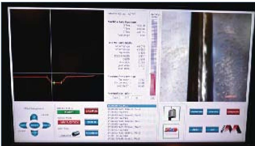
Fig. 7 — Integrated weld controller and process monitor displays.
