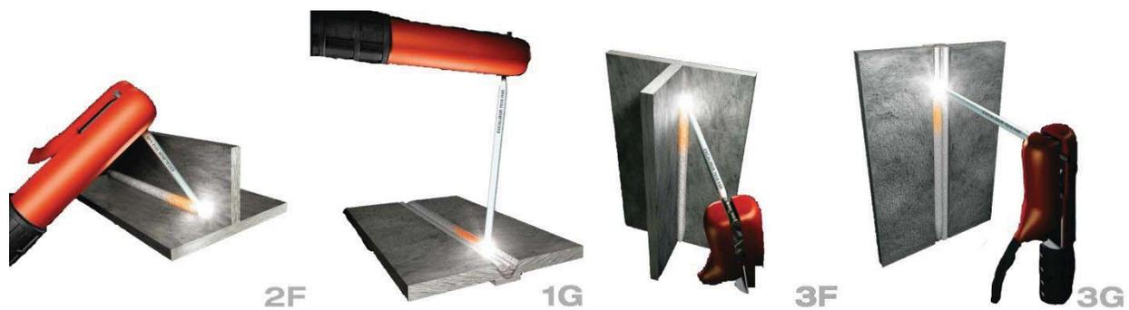
*Figure 2. The four certifiable weld positions in this study, depicted in order of increasing difficulty.*
