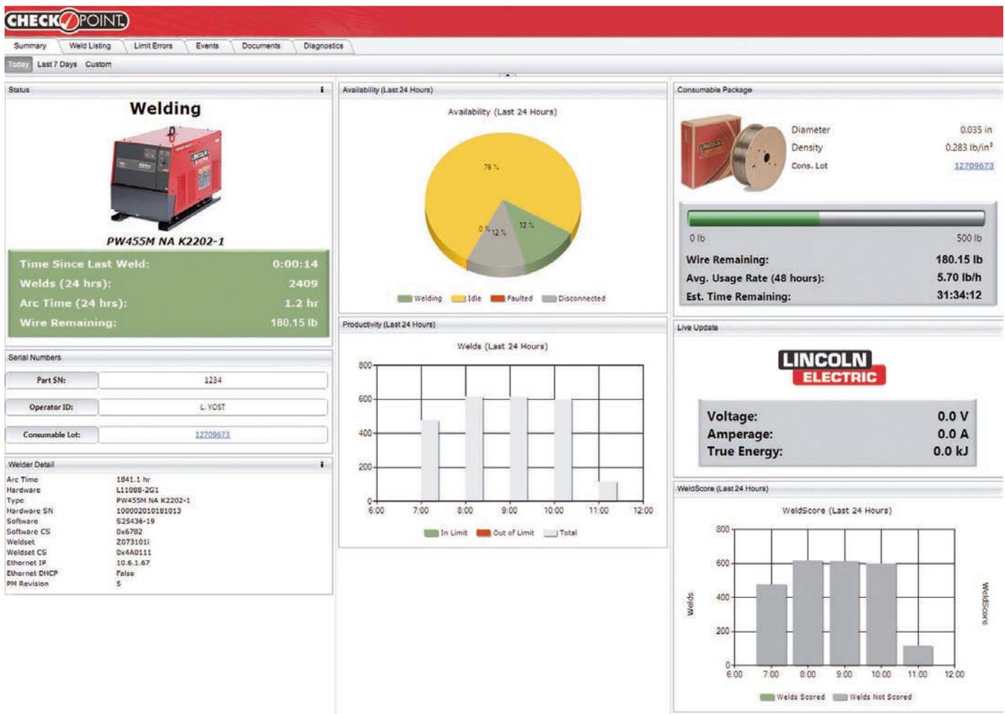
Figure 3. Cloud-based weld monitoring tools, such as Checkpoint™ Production Monitoring, simplify data collection, tracking and reporting.
