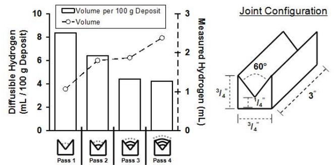
Figure 4. Diffusible hydrogen in various layers of multiple-pass welds.
