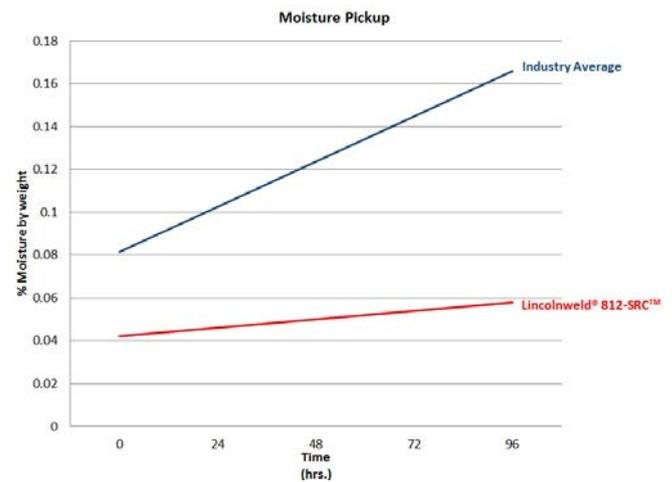
Figure 5. Low initial moisture and low moisture pickup provide low risk of delayed cracking.
