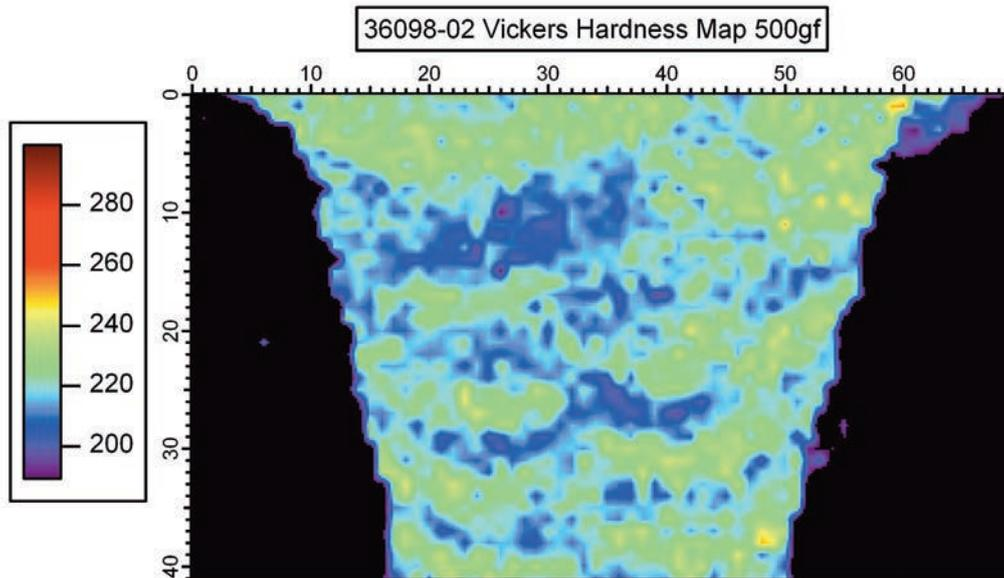
Figure 2. Weld metal hardness is reduced by heat treatment (mapped with approximately 2000 indentations).
