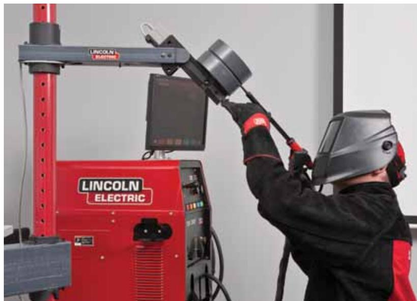
Lincoln's VRTEX 360 virtual welding solution is an ideal tool for training and qualifying pipe welders in this scarce skill.
