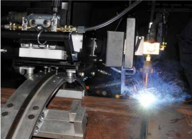
*By using a Bugo Piper-Bug with solid wire STT for the root and gas-shielded FCAW for the fill passes, 30 joints per day can typically be achieved.*
