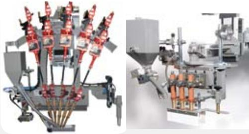
To address the special needs of multiple arc welding, it is essential to have the ability to adjust all the mechanical setup parameters.
